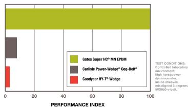
TEST CONDITIONS: Controlled laboratory environment; high horsepower misaligned 3 degrees; 5VX950 v-belt.
